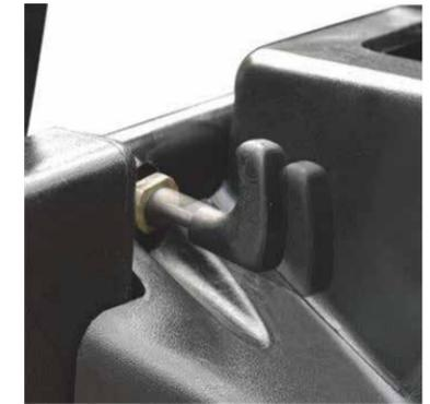
The clearance between the steering axle and support rod can be adjusted, to improve the adaptability for ground.
