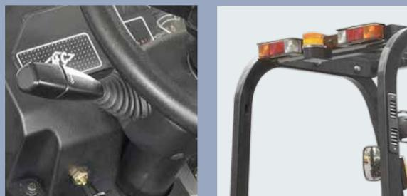
The torque converter models adopt electronic-hydraulic forward-reverse control technology, meaning less effort and less total time used during this often-performed function.
